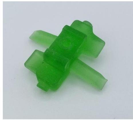
Figure 1: Repaired switch panel. Left one shows the replaced toggle Figure 2: Toggle insert. The colour only indicates the part as the replicated one
