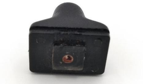
*Figure 9: Rocker switch being removed from the switch panel. The bottom is already sanded using 240 and 600 grid paper*
