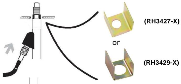
6) Place the yellow clamping "U" bracket over the mast tube and slide the aerial into the hole in the wing/fender from underneath. Replace the seal and loosely clamp the original style crown nut onto the thread at the top of the mast tube, tightening the crown nut until it begins to clamp against the "U" bracket. Please note: if the seal is in poor condition it should be replaced to prevent water ingress.
