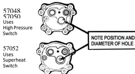
The high pressure (JLM165-X) switch or switch kit (MC1315-X + PT1032-X) is normally closed to ground to complete the clutch circuit and opens with high pressure to shut off the clutch circuit. JLM165-X or MC1315-X/PT032-X are used with replacement compressor UE43934NF.01-X & UE43934.02-X.
