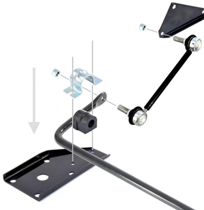
Fig. 3 Attaching the anti-roll bar, ball joints, chassis and axle plates
