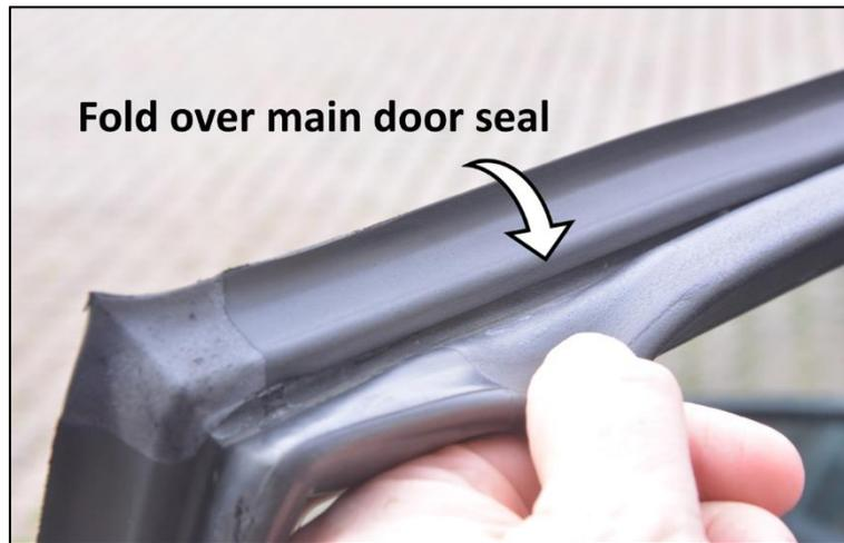
When the seal is fitted, work back along the seal with your thumb or the side of a blunt knife to ensure the seal is uniformly stuck to the frame.
