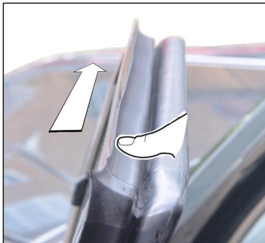
Place your thumb next to the corner so that you do not alter the alignment of the corners of the seal and frame as you stretch the seal.
