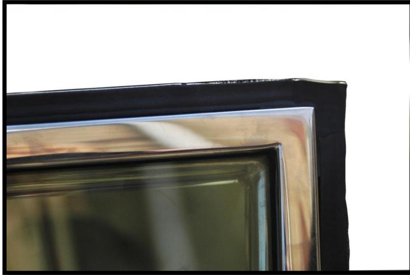
When applying the seal to the frame, stretch it moderately to place a degree of tension in the material. Putting the seal under a little tension also makes it easier to align the seal neatly with the frame. It helps to look along the frame as you fit the seal for purposes of alignment.
